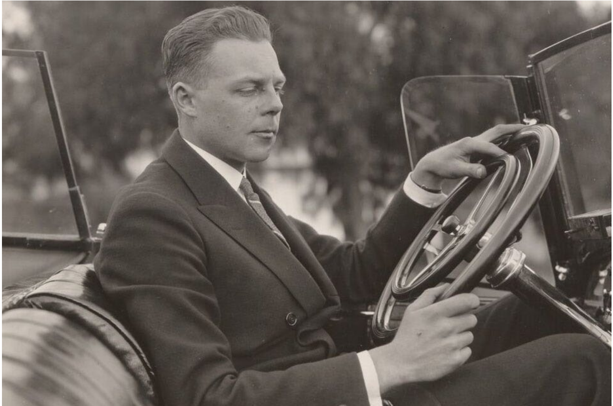
Abner Doble showing the inner steering wheel that controlled the vehicle's speed. (Photo: Doble Steam Motors Co. Photograph Collection).
